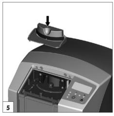
• Insert the retaining plate.
