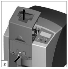
• Press the unlocking button while at the same time lifting the cover up.
