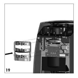
• Insert the roller locking plate.
