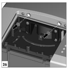
• Insert two countersunk screws with the SW 2.5 Allen key.
