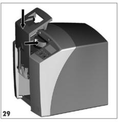
Click the retainer into place in the device and put the cover back into place at the same time.
