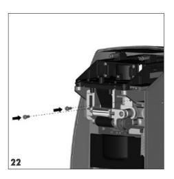
• Fix the belt drive in position using two sockethead screws and a SW 2.5 Allen key.
