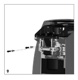
• Remove the sockethead screws from the belt drive with a SW 2.5 Allen key.
