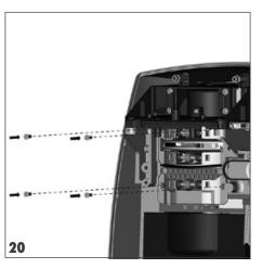
• Fix the plate in position using four counter-sunk screws and Philips screwdriver.
