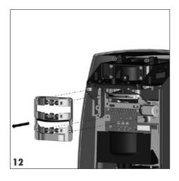
• Pull the plate forwards and outwards to remove.
