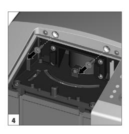
Remove two countersunk screws with the SW 2.5 Allen key.
