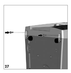
• Insert two cylinder screws on the underside with a SW 2.5 Allen key.
