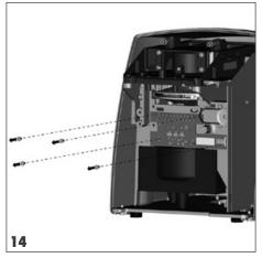
• Remove the four sockethead screws from the erasure unit with a SW 2.0 Allen key.
