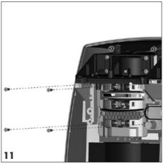
Use the Phiips screwdriver to remove four counter-sunk screws on the roller locking plate.
