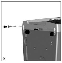
• Remove the socket-head screws underneath with the SW 2.5 Allen key.
