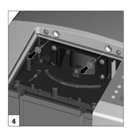
Remove two countersunk screws with the SW 2.5 Allen key.
