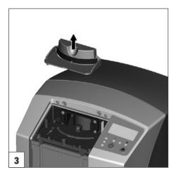
• Lift the retaining plate up and off as shown.
