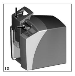
Click the retaining plate into place in the device and put the cover back into place at the same time.
